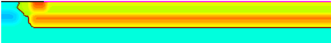
Fig. 7 Topology reduced doping profile of the LDMOS for the study of the parasitic NPN transistor. From the real structure only n-epi, sinker and buried layer are left.
