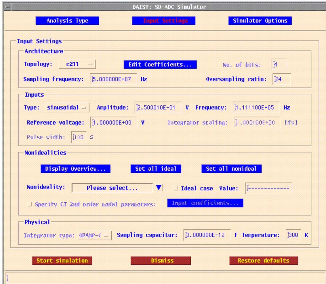
Figure 4: Input window of the \Delta\Sigma ADC simulator.
