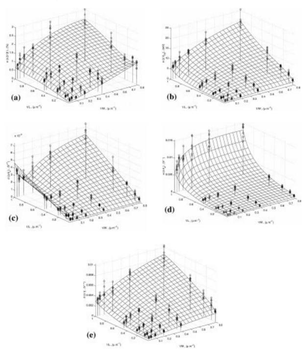
Fig. 9. Measured and fitted mismatch parameters for NMOS transistors. Diamonds are measured parameters for each transistor size and die. Surfaces correspond to fitted mathematical functions for (a)  $\sigma(\Delta\beta/\beta)$ , (b)  $\sigma(\Delta V_{T0})$ , (c)  $\sigma(\Delta\theta_o)$ , (d)  $\sigma(\Delta\theta_e)$ , (e)  $\sigma(\Delta\gamma)$ . Units for 1/W and 1/L axes are  $\mu$ m $^{-1}$ .
