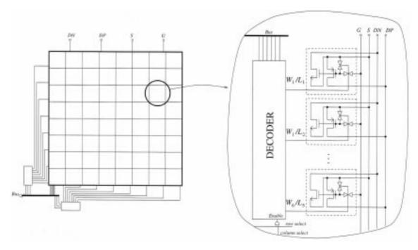
Fig. 2. Mismatch characterization chip simplified schematic.
