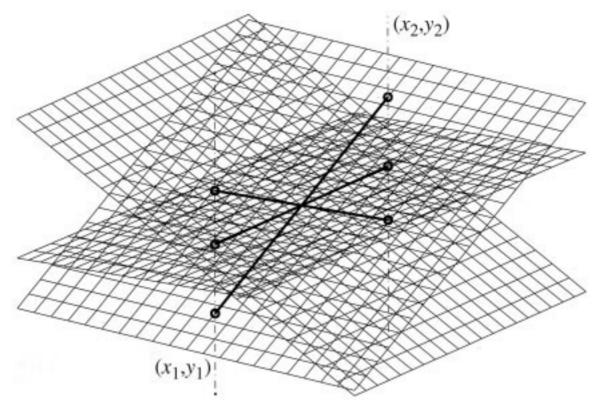
Fig. 1. Illustration of gradient-induced mismatch component for three different dies, each characterized by a gradient-plane.
