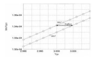
Fig. 11. Differential pair input offset voltage measurement. Curve  $I_{ds1}$  is for one of the transistors and  $I_{ds2}$  is for the other. Circles are experimentally measured points, lines are interpolated curves. Transistors are NMOS of size  $40 \, \mu \text{m} \times 40 \, \mu \text{m}$ .
